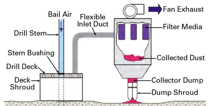
Diagram of dust control systems for rock drills, including deck shrouds for the drill bit and the discharge or dump shroud. (Illustration courtesy of NIOSH).
