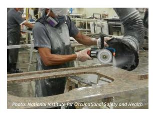
Wet methods and ventilation can reduce dust exposures
