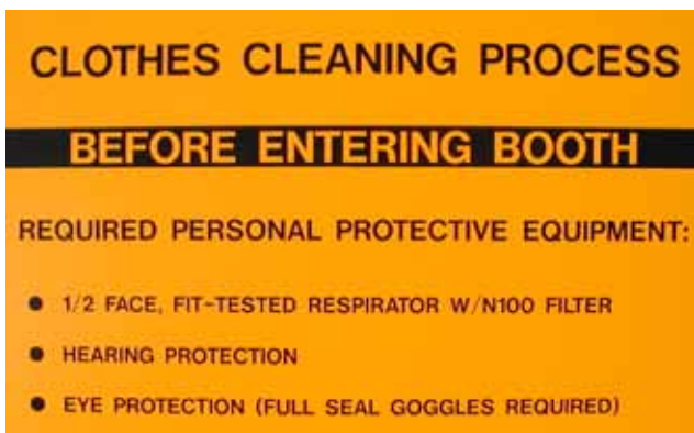
figure 6. Signage used on the door of the booth indicating the personal protective equipment required.
